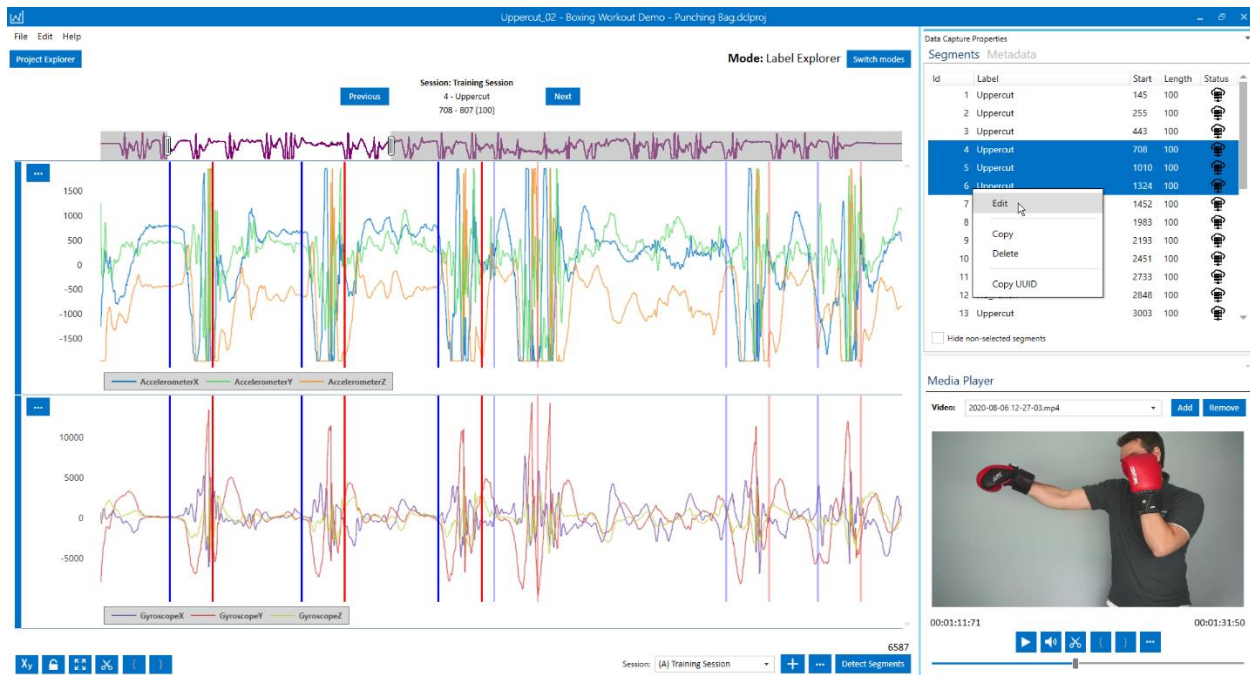
Desktop Data Capture Lab used to label and visualize raw accelerometer sensor data
