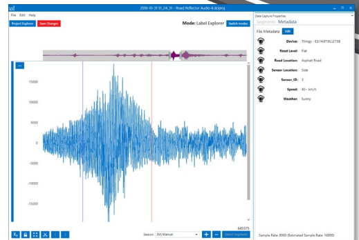
SensiML Data Capture Lab makes simple work of annotating traffic sensor data labels as necessary to train the AI model to recognize future events.
